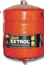
The expansion tank allows the fluid to safely expand by compressing the air in the chamber. The size of the expansion tank needed depends on the total volume of fluid, which is determined by the number and size of collectors, and the length and diameter of the pipes in the solar loop.
