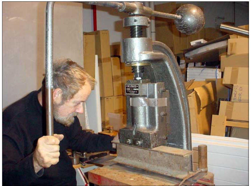
A press was used to form the channels in the aluminium fins.
