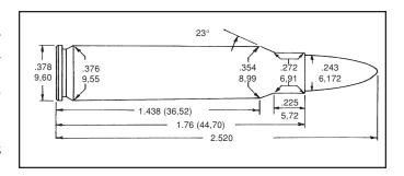
There is no SAAMI pressure limit for the 6mm T/CU. Based on the recommendations of Thompson/Center, our maximum pressures do not exceed that of the .223 Remington.
