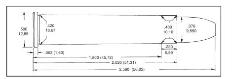
Intended to fill a gap in the cartridge line-up in Winchester's lever action rifles for large game in heavily wooded areas, the .375 Winchester ballistics are more than adequate. Unfortunately, its sales were not. Marlin also chambered their Model 336 lever action rifle for this cartridge for a time as did Ruger in the No. 3 carbine. Today, however, no rifles are produced for this cartridge.
