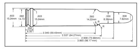
tridge for driving a heavy .30 caliber bullet very far, very fast.
