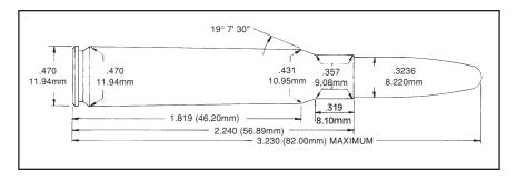
The European pressure limit for the 8x57mm is approximately 97% of the loading limit for the .30-06. This equates to a working pressure limit of about 58,200 P.S.I. The performance of the 8mm Mauser is excellent when loaded to its full potential. This data should only be used in rifles that have been determined to be safe by a competent gunsmith and that are known to have "JS" bore dimensions (.323" groove diameter).
