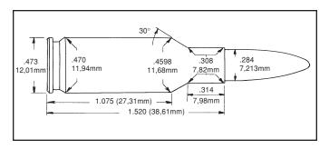
The 7mm BR is based on a thin-walled version of the .308 Winchester case that utilizes a small primer pocket and is shortened to 1.5".
