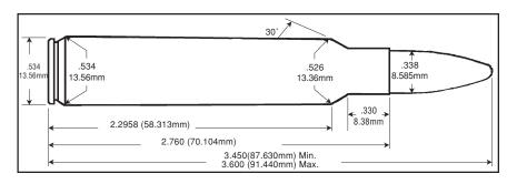
SAAMI Maximum Average Pressure is set at 65,000 P.S.I. Please use starting loads for this cartridge as reference ammunition was not yet available when we developed the following data.
