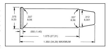
This cartridge is the .32 S&W Long lengthened by 0.155". Any revolver cham-
