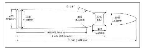
As a result of ballistic experiments in Europe, the U. S. Army modified the .30-03 cartridge by shortening the neck 0.070" and loading a short pointed bullet weighing 150 grains to a muzzle velocity of 2,700 FPS. This cartridge then became known as the Caliber .30, Model of 1906 or simply the .30-06 Springfield.
