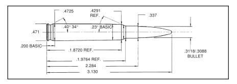
the .303 British cartridge and uses the same diameter bullets. However, the 7.7mm Arisaka is a rimless case whereas the British round is rimmed.
