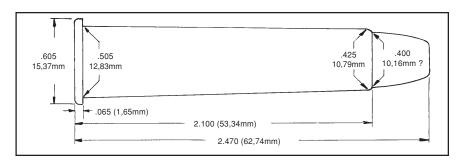
The .40-65 was loaded with both black and smokeless powder and remained listed in Winchester catalogs until about 1935. The .40-65 Winchester is essentially the .45-70 Government cartridge necked down to .40 caliber. The purpose behind this cartridge was to increase the power available in Winchester's lever action rifles thus making them more competitive with their single-shot rivals.
