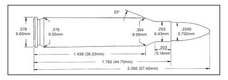
in chamber dimensions, principally in the chamber throat, have occurred since the 5.56 cartridge was adopted, the latest version to accommodate the heavier SS109 projectile.
