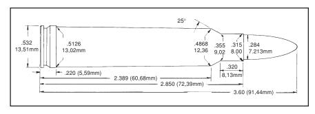
This cartridge is best suited for single shot rifles such as the Ruger #1 or Browning Model 78, which permit proper seating of the heavier projectiles. When heavy bullets are loaded in this cartridge and seated to an overall length that will permit them to function in the magazine of a Remington 700, the rear of the bullet protrudes rather deeply into the powder space producing large variations in pressures and velocities.
