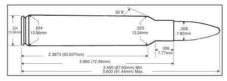
ume by using a necked down .404 Jeffery case which provides about 10% more volume than other .300 Magnum cartridges. This extra volume allows for a higher propellant charge weight which results in higher velocities.
