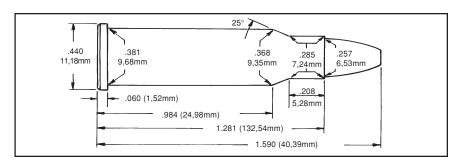
Ruger revolvers chambered for this cartridge never materialized due to technical problems associated with setback of the bottle-necked case when the cartridge is fired in a revolver.
