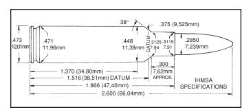
There is no SAAMI pressure limit for the 7mm IHMSA. Based on the strength of the Wichita bolt action handgun, the maximum loads listed below do not exceed that of the 7mm-08 Remington.
