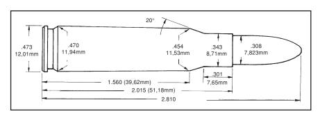
The .308 was the result of the military's experiments to retain the power of the .30-06 cartridge in a smaller package. The advent of Winchester ball powder permitted loading the 7.62x51mm to equal the velocities of .30-06 service ammunition.
