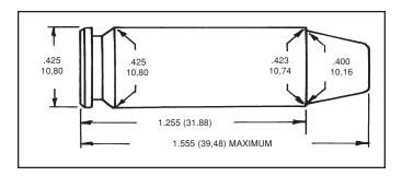
This cartridge is a lengthened 10mm Auto and is loaded to pressure levels similar to the .44 Magnum for use in the IAI handguns.
