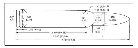
The .416 Weatherby factory ammunition produced 60,000 P.S.I. in our test barrel. These loads to not exceed that pressure.
