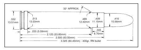
that .411" diameter bullets feed through the magazine of the Voere rifles more reliably than .416" bullets used in the same cartridge. Accurate **2460** and **2520** are the best all-around powders.
