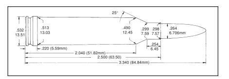
designed to produce what Winchester hoped would be the ultimate open-country hunting cartridge for deer-sized big game. To accomplish this feat of engineering, Winchester's ballisticians utilized a 2-diameter bullet with only the section aft of the cannelure being full groove diameter.
