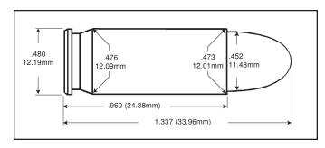
the pressure limit for this cartridge has been set at 40,000 C.U.P. as well. The loading data shown below does not exceed this limit. These loads are considered maximum by the technical staff at Accurate Arms Company. Never exceed these loads. Never shoot .460 Rowland ammunition in any firearm not designed for it's use.
