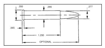
There is no SAAMI pressure limit for the .270 R.E.N. The maximum loads listed below are approved by the manufacturer of the Merrill single shot pistol, Jim Rock.
