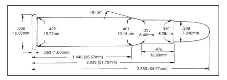
let and 30 grains of smokeless propellant. Muzzle velocities approached 2000 FPS. Winchester later adapted the Model 54 bolt action to handle the .30-30.
