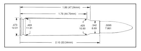
sporting ammunition and produced rifles chambered for this cartridge until about 1936. Similar in power to the .308 Winchester, the 7.65 Mauser is adequate for hunting most big game in North America. Both ammunition and brass are available from Norma.
