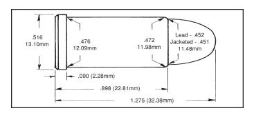
a rimmed version of the .45 ACP which eliminated the need for using the pesky clips in these revolvers. The .45 AR was also loaded with a lead bullet to reduce wear on the shallow rifling used in these revolvers.
