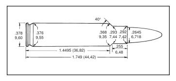
The 6.5 T/CU should be adequate for small game and varmints at ranges up to 200 yards. There is no SAAMI pressure limit for the 6.5 T/CU. Based on the recommendations of Thompson/Center, these loads are limited to the same pressures as the .223 Remington cartridge.
